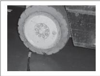
Avoid compression of the cable as may be caused by running over with any wheeled vehicles such as fork lifts, carts, vans, dollies, etc.
