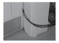
• During operation, **avoid** bending cable around sharp edges such as door jams and furniture.
